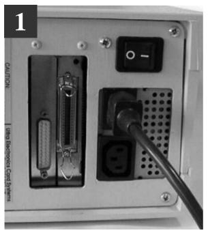
Switch the printer OFF. Locate the Parallel Interface connector on the rear panel.
